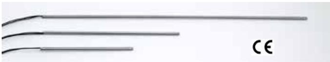
Closed end 1/8 inch (3.175 mm) diameter stainless steel tube. Available in three lengths: 4, 6 and 12 inch (101, 152 and 304 mm). Teflon insulated 24 gage leads. Inserts into a Pete's Plug or CF916 fitting (below). Suitable for HVAC and general temperature applications.
