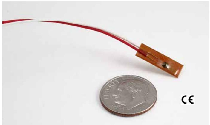
The PT510 and PT520 Temperature Sensors consists of a thin-film platinum element encased in a high temperature laminate. The PT520 can operate at continuous temperatures of up to 260°C. The PT510 includes an adhesive backing for easy mounting. A maximum of four PT510 / PT520 sensors may be connected to one XR450 Pocket Logger.
