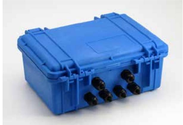
Rugged molded case withstands all weather conditions. Features a hinged cover, continuous neoprene o-ring seal, quick release latches, and fold-up carrying handle. Six feed-through cable glands accept cable diameters up to 0.25" (6.3 mm). Can be padlocked for security.
