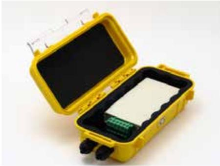
Rugged molded case withstands all weather conditions. Features a hinged cover, quick release latch, continuous rubber seal and two cable fittings. Fittings accept cable diameters up to 0.25" (6.3 mm). Available in Black only. Yellow case pictured above is no longer available.
