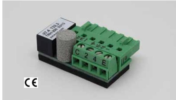
perature and humidity range (see below). Two channels are available for other PACE sensors, 0-5 vdc or resistive signals.
