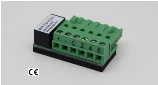
Four millivolt plug-in modules are available, each with a different millivolt range. Three of the modules (Mvt-11b, Mvt-22b, Mvt-50u) also accept a Thermocouple (Type J, K, N, R, S, T, B, C or E). A built-in, precision thermistor provides ambient temperature readings and for thermocouples, cold junction compensation.
