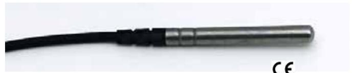
Rugged stainless steel probe, 6 mm (0.236") diameter and 50 mm (approx 2 inch) length with 6.1 meter (20 ft) cable. TPE jacketed cable with a diameter of 3.3 mm (0.13"), a round cross section and 24 gage, polypropylene insulated leads. Suitable for immersion, HVAC, and soil burial applications. Probe's cable is not recommended for immersion in fuels (fuel splashing on cable is OK).
