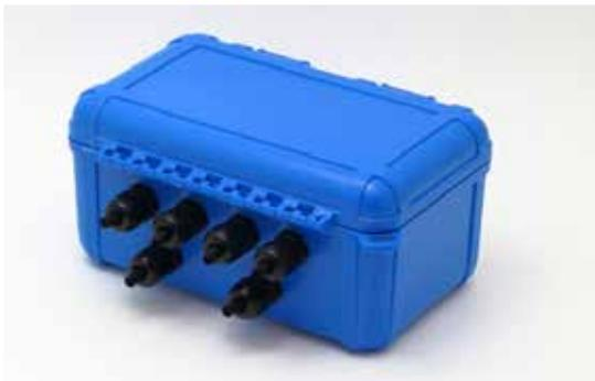
Rugged molded case withstands all weather conditions. Features a hinged cover, continuous neoprene o-ring seal and two quick release latches. Six cable fittings installed on side of case. Fittings accept cable diameters up to 0.25" (6.3 mm).
